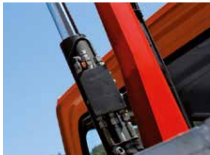
Hydraulic overload protection In-built safety function
