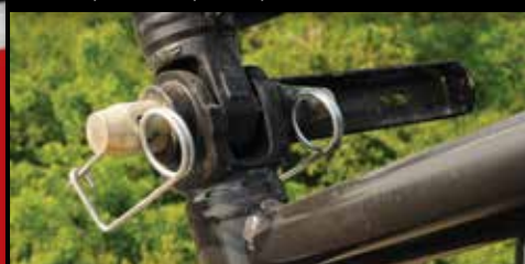
Double-tapered boom pin with pin catcher
