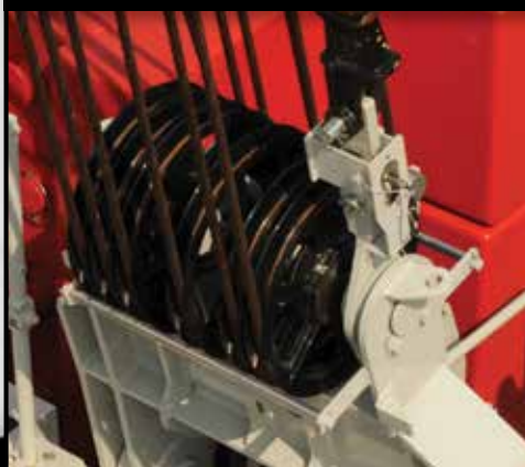
In-line boom suspension load cell
