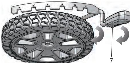
1. Pull the height adjustment lever (7) rearward to increase the cutting height.
