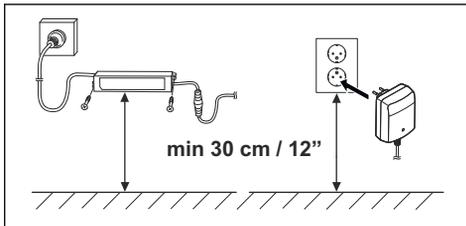
5. Connect the power supply cable to a 100-240V power outlet.
