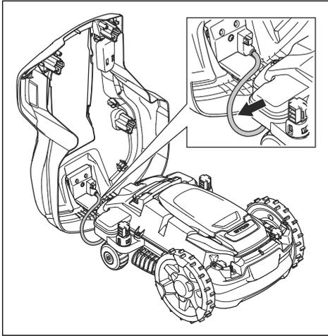
**Note:** Make sure that the grommets for the charging cable are correctly installed to seal against moisture after you remove the body of the product.
