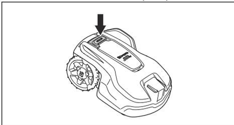
2. Push the **ON/OFF** button for 3 seconds and make sure the product is switched off. Check that the indicator lamp on the keypad is not lit. This means that the product is disabled. Refer to *To use the ON/OFF button on page 31*.
