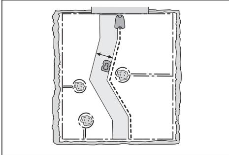
The corridor width is adjusted automatically. If it is necessary to adjust the corridor width manually for the product to operate satisfactorily, you can set the corridor width between 1-9. The factory setting is 6.
