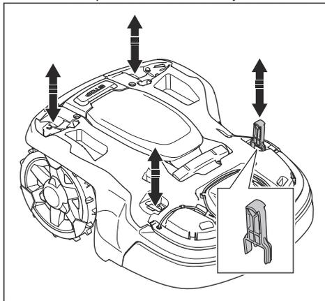
5. Push the maintenance tool down in 1 of the 4 positions, and pull the body up.
