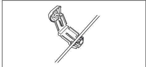
3. Close the connector with a pair of pliers.
