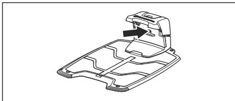
2. Check that the boundary wire connections to the charging station are properly connected and not damaged. Check that the indicator lamp in the charging station is still flashing blue.
