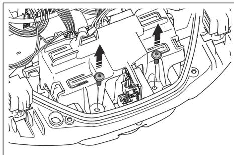
7. Push to detach the clips and lift up the battery holder.
