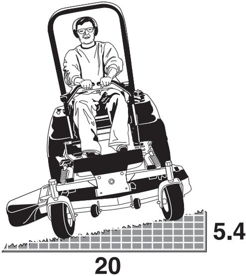
Operation on slopes can be dangerous. Using the unit on a slope that is too steep where you do not have adequate wheel traction (and control) can cause sliding, loss of steering, control, and possible rollover. You should not operate on a slope greater than a 5.4 foot rise over a 20 foot length (15 degrees).
