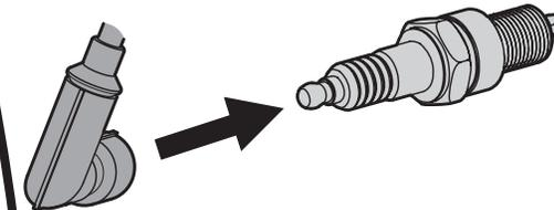
Make sure the spark plug boot is connected to the spark plug before attempting to start.
