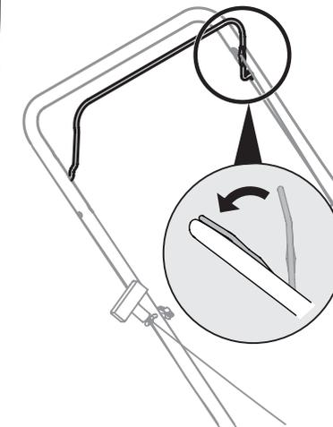
While standing behind the machine, pivot the Blade Control Handle against the upper handle.
