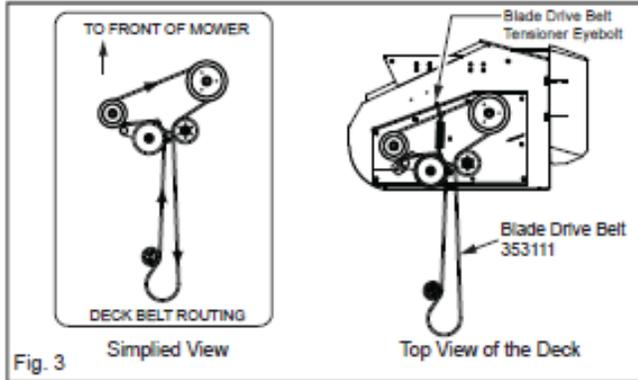
Approximately 1/8" stretch between coils. Turning the nut on the eyebolt clockwise will decrease tension. When installing a blade drive belt please refer to figure 3 for routing the blade drive belt. The pump belt
