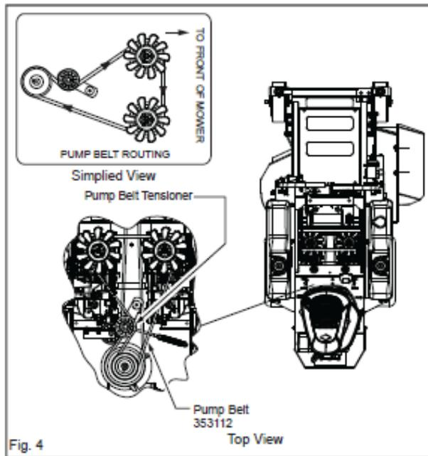
may be accessed from under the rear chassis. The pump belt is removed by unhooking the tensioner spring to provide slack in the belt for removal. When installing a pump belt please refer to figure 4 for the routing of the pump belt.
