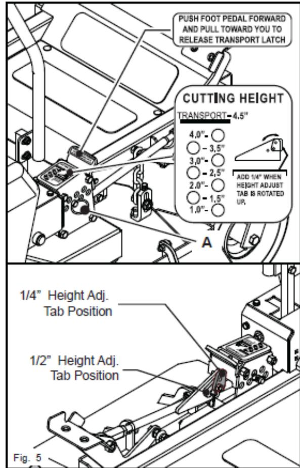
Height of cut positions are drilled at 1/2 inch increments. To add 1/4 inch to the setting you must first remove the #4 hairpin cotter, pull pin and rotate the tab to the vertical position. The foot pedal must be depressed slightly in order to replace the pin in tab. See Fig. 5
