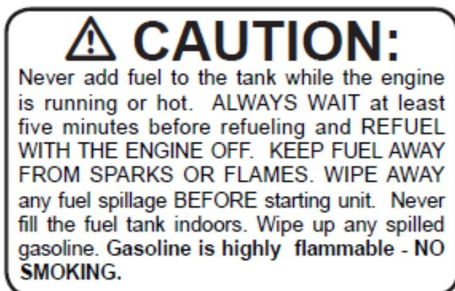
7. Handle gasoline carefully, Use an approved gasoline container. Fill the fuel tank, to within 1" from the neck, with good quality unleaded gasoline.
