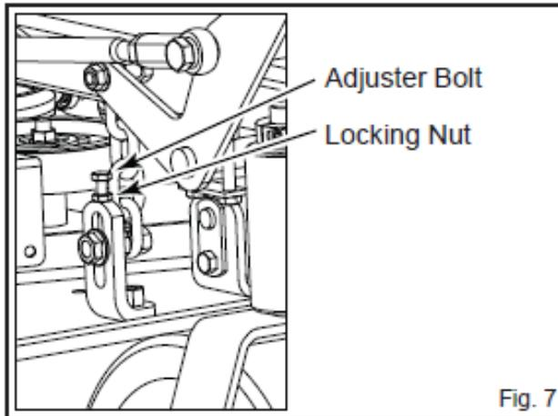
Always maintain at least a 1/7 inch of deck pitch from front to back. Also all four chains must support the deck equally or must have equal tension on them.
